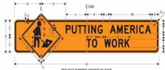
PROJECT FUNDING SOURCE PLAQUE
